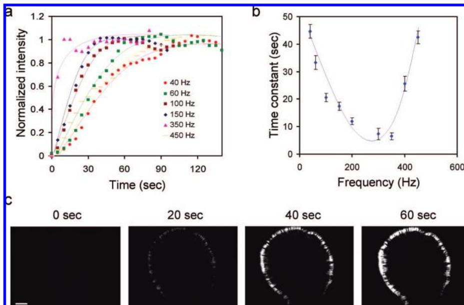
**Figure 3.** Kinetics of the QD concentration process at the edge. (a) Kinetics of the concentration process at different frequencies. The applied voltage was  $10 V_{pp}$ . (b) Frequency dependence of the concentration process at  $10 V_{pp}$ . The smallest time constant for the concentration process is approximately at 300 Hz. (c) Video time series of the concentration process ( $8 V_{pp}$ , 400 Hz). Scale bar is  $100 \mu\text{m}$ .
