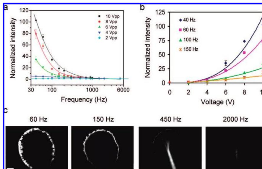
**Figure 2.** Electrokinetic concentration of QDs at the edge of the inner electrode. (a) Frequency dependence of the concentration process at different voltages. (b) Voltage dependence of the concentration process at different frequencies. The scaling exponents were determined to be  $2.93 \pm 0.26$  (at 40 Hz),  $2.63 \pm 0.20$  (at 60 Hz),  $2.12 \pm 0.29$  (at 100 Hz), and  $1.47 \pm 0.38$  (at 150 Hz). (c) Concentration of QDs at different frequencies. Scale bar is 100  $\mu\text{m}$ .
