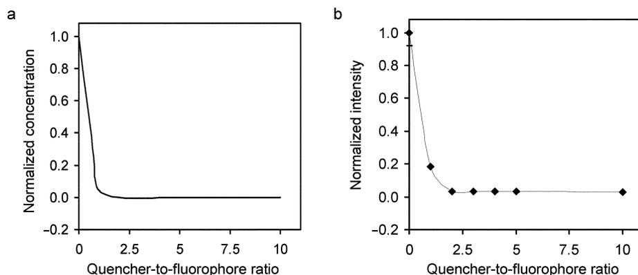
**Fig. 4** Optimization of the quencher-to-fluorophore ratio. The equilibrium concentration of the free fluorophore probe determined by (a) the equilibrium analysis and (b) experimental investigation. The concentration of the fluorophore probe is 40 nM and the concentration of the quencher probe is adjusted to obtain different quencher-to-fluorophore ratios. Error bars representing the standard deviation are not shown as they are smaller than the symbols themselves.
