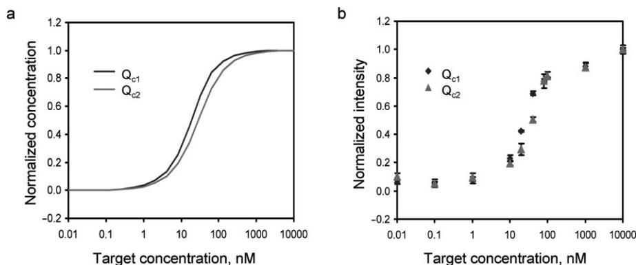
**Fig. 2** Effects of the quencher length on the molecular assay shown by (a) the equilibrium analysis prediction and (b) experimental investigation. Quencher probes are of length 12 ( $Q_{c1}$ ) and 16 ( $Q_{c2}$ ) nucleotides respectively. The probes were employed in samples with a 60nM concentration with 20nM fluorophore probes to gauge the effect of the quencher probe design on the system sensitivity. Data represents mean  $\pm$  standard deviation.
