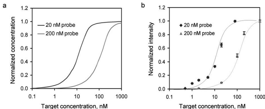
**Fig. 3** Tunable dynamic range of the molecular probe assay determined by (a) the equilibrium analysis and (b) experimental investigation. Fluorophore probe concentrations of 20 and 200 nM and quencher probe concentrations of 40 and 400 nM were used, respectively. Error bars represent the standard deviation.
