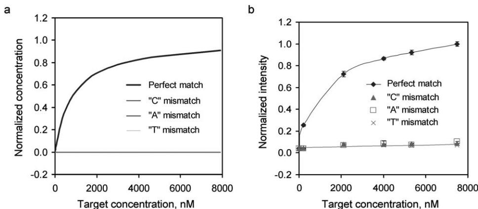
**Fig. 5** Detection of single-base-mismatches using the molecular probe biosensor. The fluorescence response of the assay determined by the (a) equilibrium analysis and (b) experimental investigation. The three mismatch targets show insignificant increases in the equilibrium analysis and cannot be distinguished in the graph. The overall signal-to-noise ratio of the assay is 24 and the selectivity for single-base-mismatch is 14. Error bars represent the standard deviations.
