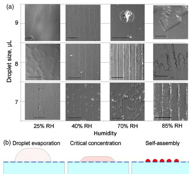
FIG. 3. (Color online) (a) EAPL of SELP at different humidity and initial droplet volume. Scale bars: 50 μm. The droplet covers an area of ~17 mm<sup>2</sup>. (b) Schematics illustrating the evaporation-induced assembly process. Author complimentary copy. Redistribution subject to AIP license or copyright, see <http://apl.aip.org/apl/copyright.jsp>
