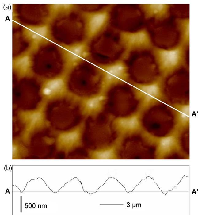
FIG. 2. (Color online) (a) AFM characterization of the self-assembled SELP structure as in Fig. 1(f). (b) Section analysis of the structure.
