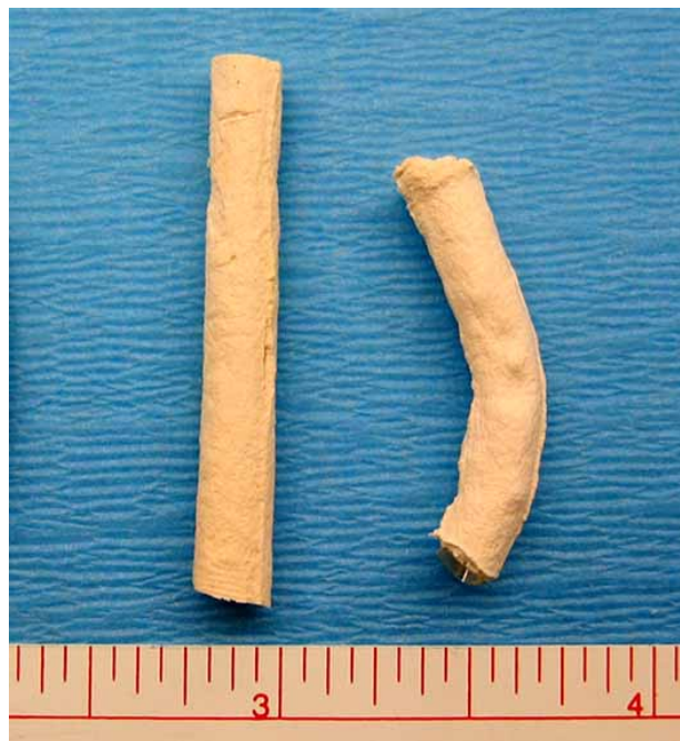
Fig. (2). Soft and elastic poly (diol citrate) biphasic scaffold consisting of a non-porous lumen and porous outer phase for small diameter blood vessel tissue engineering.
