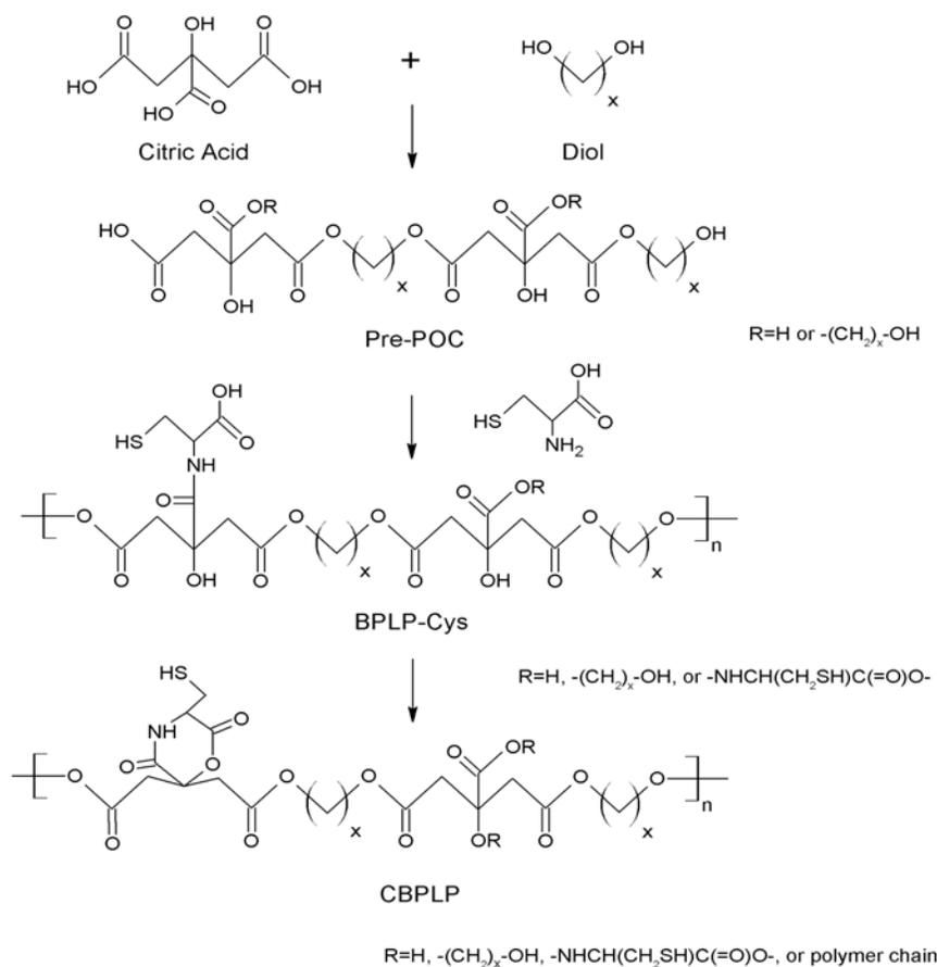
**Fig. (8).** Representative synthesis schematic of biodegradable aliphatic photoluminescent polymer reacted with L-cysteine (BPLP-cys).
