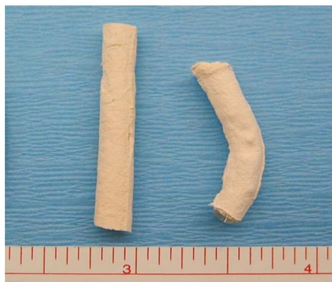
**Fig. (2).** Soft and elastic poly (diol citrate) biphasic scaffold consisting of a non-porous lumen and porous outer phase for small diameter blood vessel tissue engineering.
