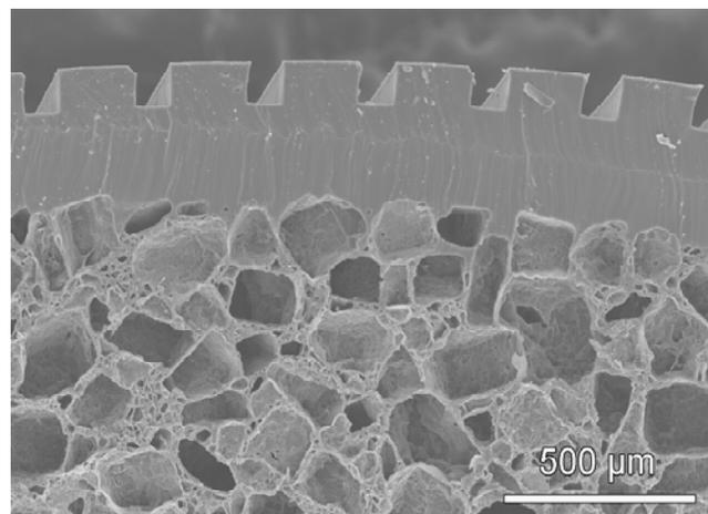
**Fig. (6).** Scanning electron microscope picture of poly (alkylene maleate citrate) scaffold cross section using microelectromechanical (MEMS) technology. Soft and elastic microchannels have been incorporated on traditional particulate leached scaffolds.
