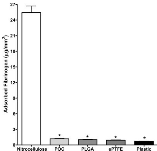
**Figure 7.** Analysis of fibrinogen protein adsorption to POC, PLGA, ePTFE, and untreated plastic. Nitrocellulose membranes serve as positive control surface for maximal fibrinogen absorption. \*Corresponds to a  $p < 0.001$  in comparison with nitrocellulose control.  $N = 5 \pm \text{SEM}$ .
