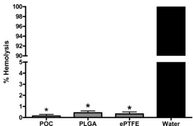
**Figure 6.** Hemolysis of red blood cells following incubation of whole blood with POC, PLGA, and ePTFE. Blood samples exposed to complete hemolysis with water were used to normalize the data. \*Corresponds to a  $p < 0.001$  in comparison to control.  $N = 15 \pm$  SEM.
