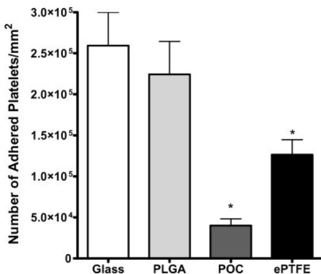
**Figure 2.** Quantification of platelet adhesion on glass, PLGA, POC, and ePTFE as determined by quantification of LDH activity. For each sample, platelet attachment was normalized by area (mm<sup>2</sup>). \*Corresponds to a  $p < 0.05$  in comparison to platelet adhesion to glass.  $N = 21 \pm \text{SEM}$ .
