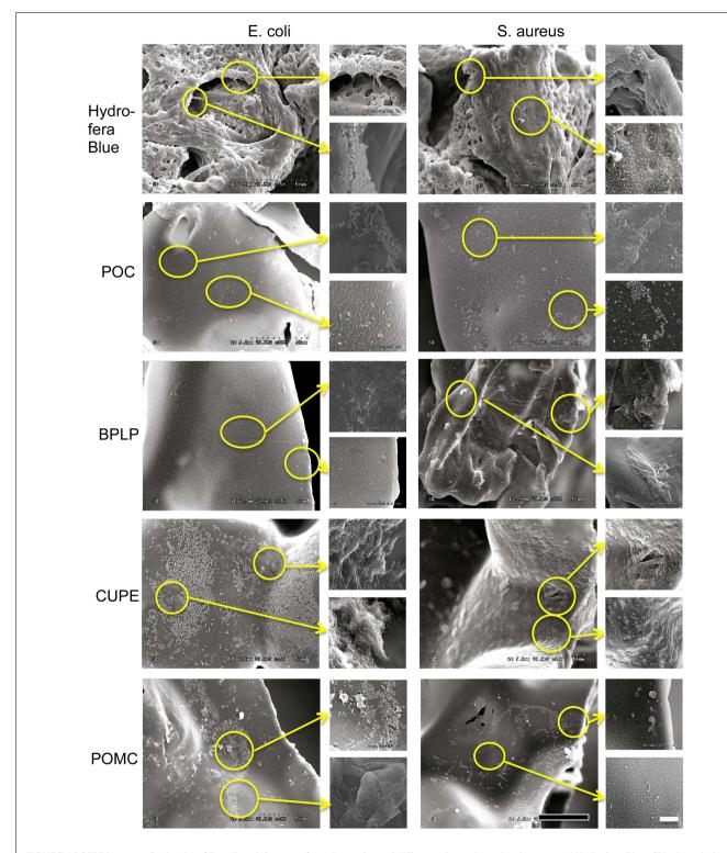
FIGURE 6 | SEM images of microbes (*E. coli* and *S. aureus*) on the surface of different citrate-based polymers and Hydrofera Blue. (Black scale bar for  $800 \times \text{magnification} = 50 \,\mu\text{m}$ ; White scale bar for enlarged  $4000 \times \text{magnification} = 10 \,\mu\text{m}$ ).
