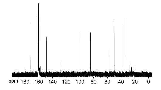
**Figure S22.** <sup>13</sup>C NMR (DMSO-d<sub>6</sub>) spectrum of CA-Cysteamine. δ 171.5, 160.6, 148.7, 101.3, 84.7, 57.5, 49.9, 34.0.
