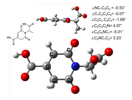
**Figure S14.** Spatial conformations of CA-Ala. Dihedral angles of any four atoms are listed on the right side.
