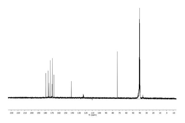
**Figure S36.** <sup>13</sup>C NMR spectrum of CA-Gly. δ 175.3, 172.0, 169.0, 166.7, 140.9, 72.8, 39.8, 34.9.
