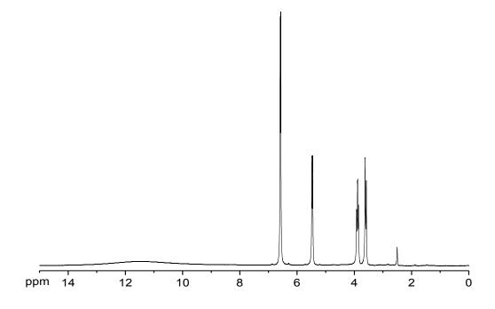
**Figure S16.** <sup>1</sup>H NMR (DMSO-d<sub>6</sub>) spectrum of CA-Cys. δ 6.58 (d, 1H), 5.48 (d, 1H), 3.90 (t, 1H), 3.60 (d, 2H).
