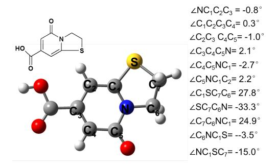
**Figure S23.** Spatial conformation of CA-Cysteamine. Dihedral angles of any four atoms are listed on the right side.
