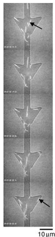
Fig. 3. Rectifying microtubule movements by arrowhead structures. A microtubule can be seen moving upward inside the arrowhead, bumping into the photoresist wall, and being redirected back into the channel. Rhodamine-labeled microtubules and SU-8 channel walls were imaged using simultaneous fluorescence and differential interference contrast microscopy.
